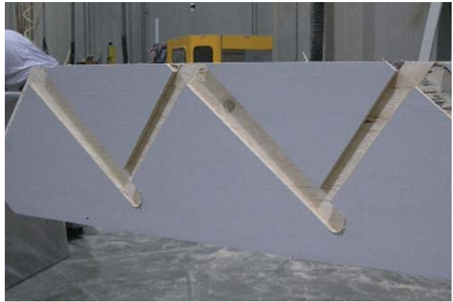
Typical Master Stair stair stringer component
